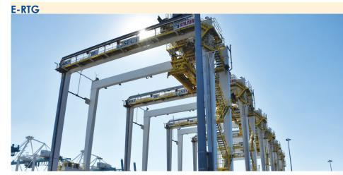
South Florida Container Terminal received 6 Electric Rubber-Tyred Gantry cranes at the beginning of 2020. Phase 1 completed in April 2021 with final Phase completion estimated to be in Q4 of 2023. RTGs greatly increase efficiencies while decreasing emissions. The electric power system removes the need for engine component maintenance, lowering downtime and reducing maintenance costs.
