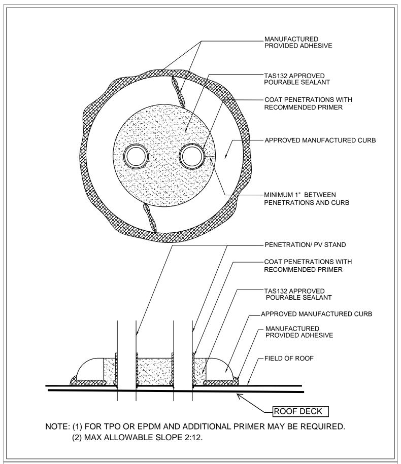
DETAIL "C" MANUFACTURED CURB LOW SLOPE
